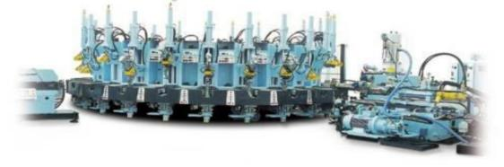
Fig. 2: Direct injection process moulding machine.
