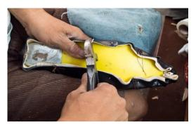
Fig. 1: Lasting process.
