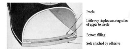
Fig. 5: Cemented lasting construction.
