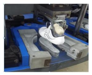
Fig. 8: TS 700 JR directly injected by TPR.
