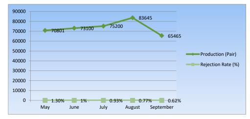
Fig. 15: Graphical representation of rejection data for sample TS 700.
