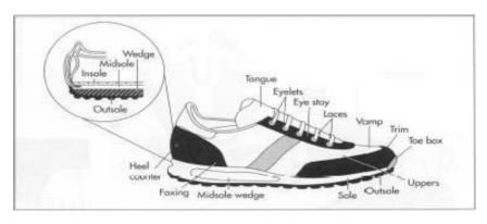
Fig. 4: Cemented lasted full shoe.
